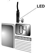
Test the Home Producer 8. The Command Center will convert the RF signal from the Home Producer 8 into and IR signal and transmit that signal to your component through the IR signal extension cord.
